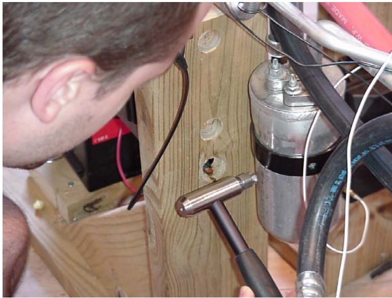
Figure 4-12: Performance of modal test
