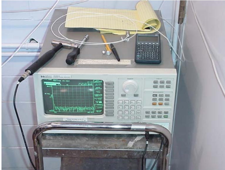
Figure 2-4: Impact hammer, accelerometer, and signal analyzer
