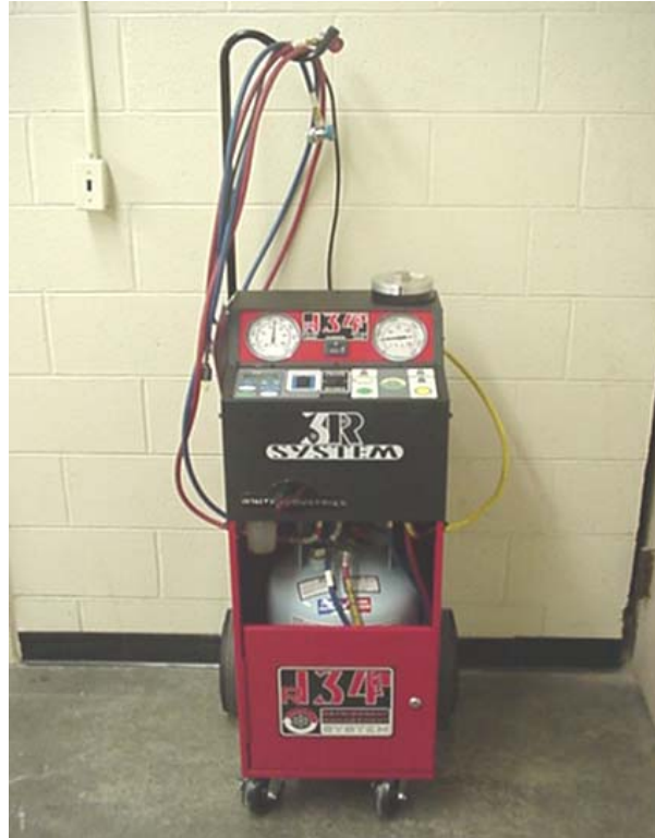
Figure 4-8: Refrigerant management system
