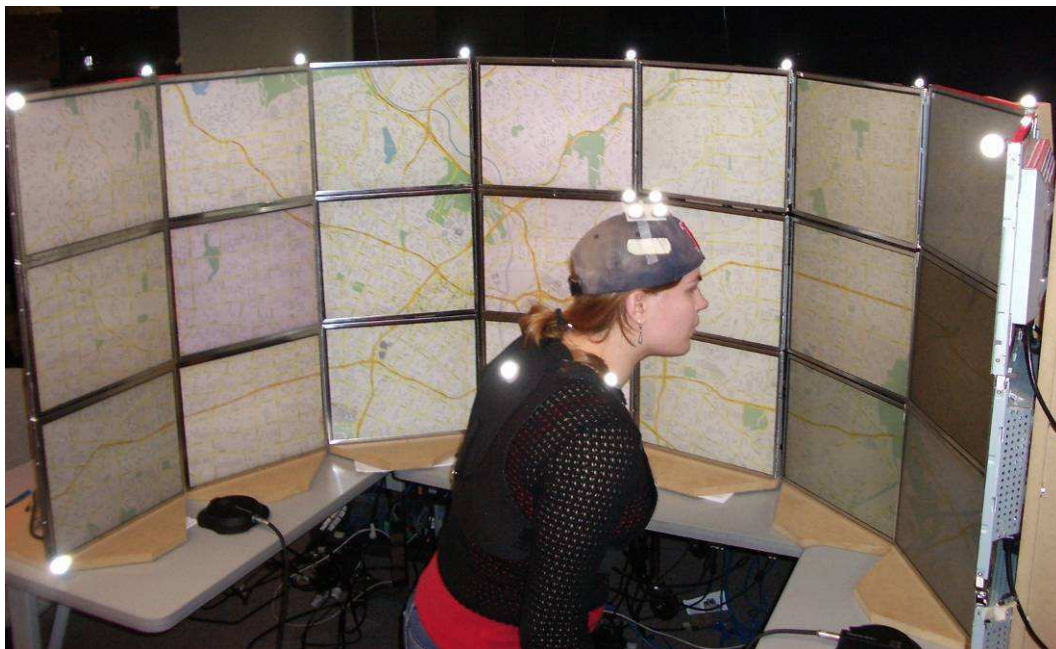
Figure 1.1: Twenty-four monitor display in the curved form with Vicon motion trackers
