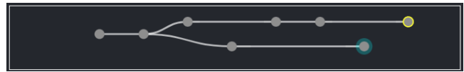
Figure 3: A live coder can create a branch from any node by clicking a node and revising its code. Here, the second node from the left has two branches (e.g., two musical variations). The horizontal placement of the nodes corresponds to their creation time, with newer nodes appearing to the right. The selected node (highlighted yellow) is the node that was added most recently.
