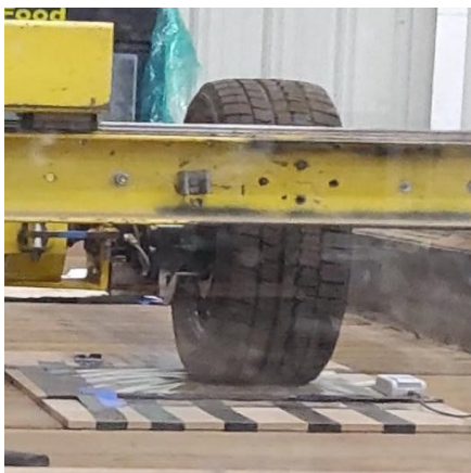
Figure 6: Squeezing of the pressure distribution setup when a tire is rotating with 12% slip ratio
