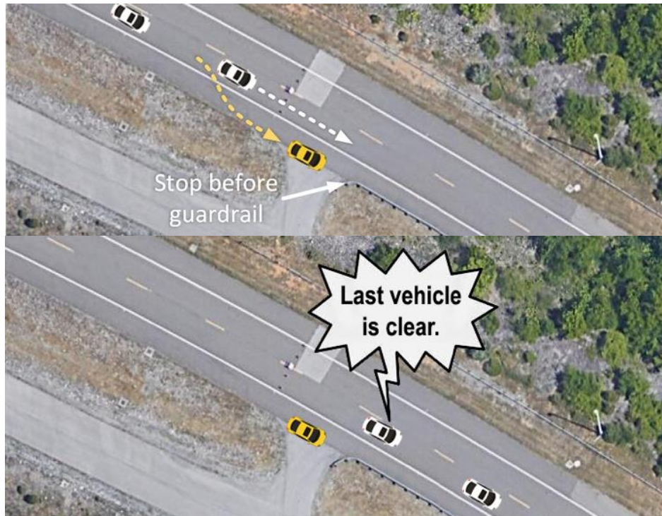
Figure 16. Diagram. Use Case Scenario 2: Lead vehicle pull-over configuration (downhill).
