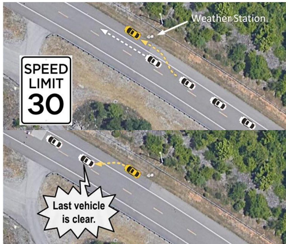
Figure 15. Diagram. Use Case Scenario 2: Lead vehicle pull-over vehicle configuration (uphill).
