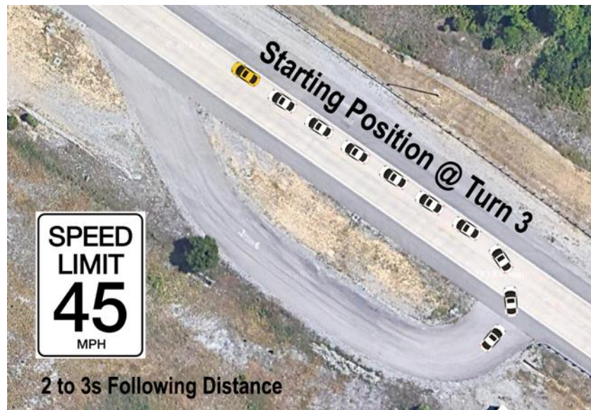
Figure 14. Diagram. Use Case Scenario 1: Free-flow vehicle configuration.
