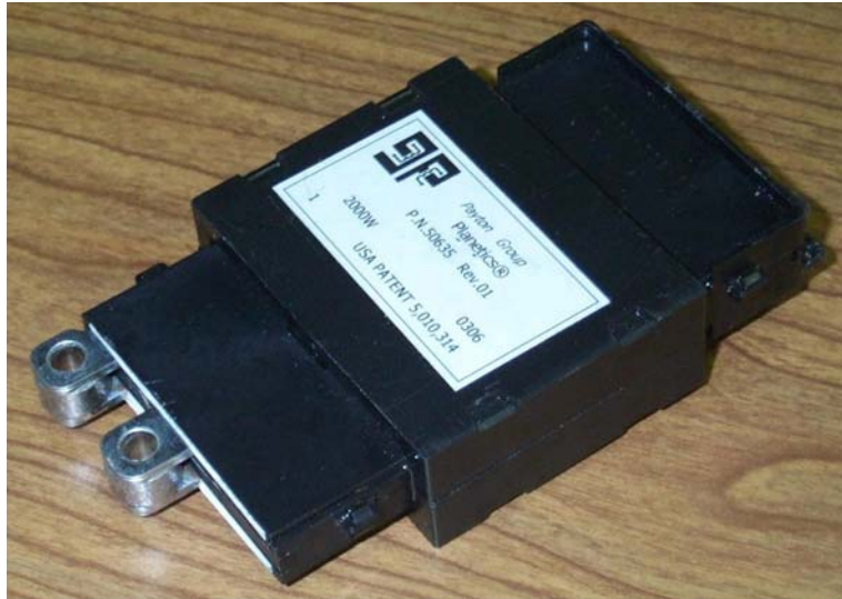
Figure 2-6. 2kW 1:6:6 planar transformer
