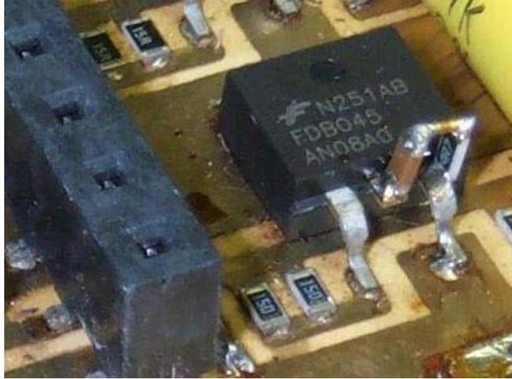
Figure 4-5. Low inductance device mounted snubbers
