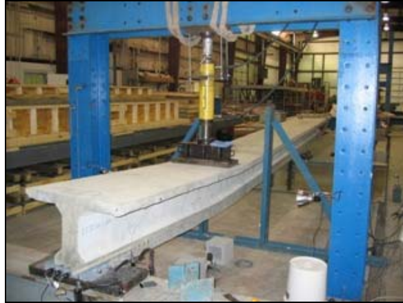
Figure 3.30. Single Point Bending Test Setup
