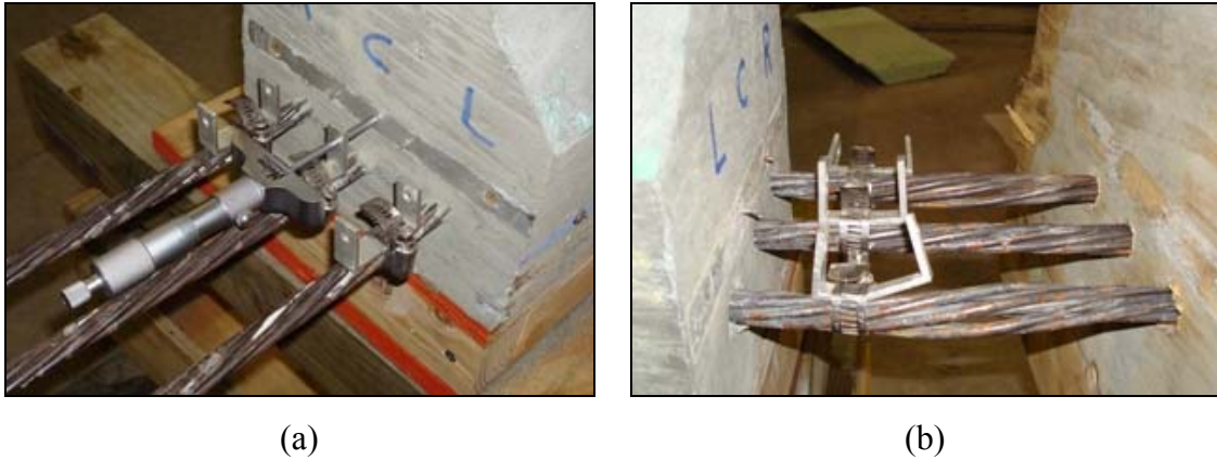
Figure 3.29. End-slip Measurements Setup
