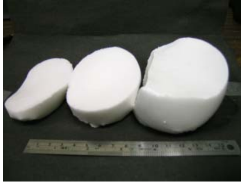
Figure 3-4. Picture of the three soft-tissue mimicking phantoms made of Zerdine™ with thicknesses of 12mm, 23mm and 31mm.
