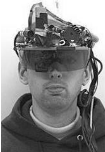
Figure 1. A prototype head-mounted display for augmented reality applications ( http://www.wearcam.org/head-mounted-displays.html ).
