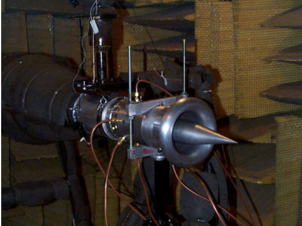
Figure 3.5: Boeing Translating Inlet during Testing
