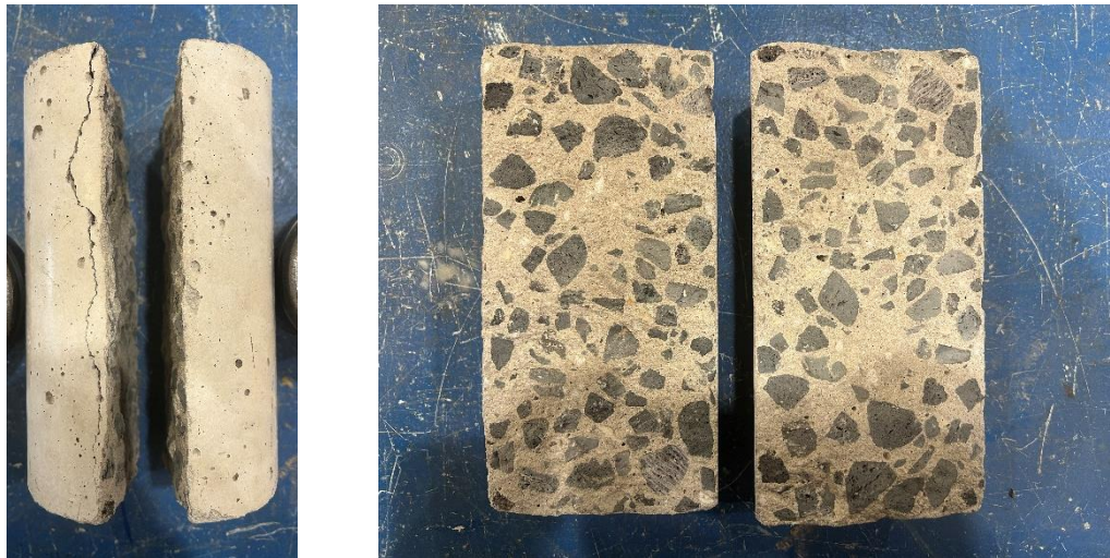
Figure 6-12. Cracks Forming Through Aggregate in LWC.
