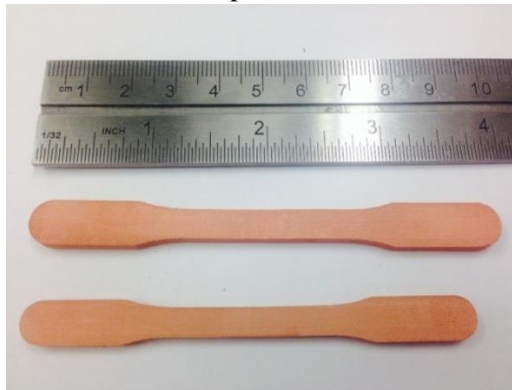
Figure 2.11 Tensile test specimen sintered at 1060 °C (top) and 1080 °C (bottom)
