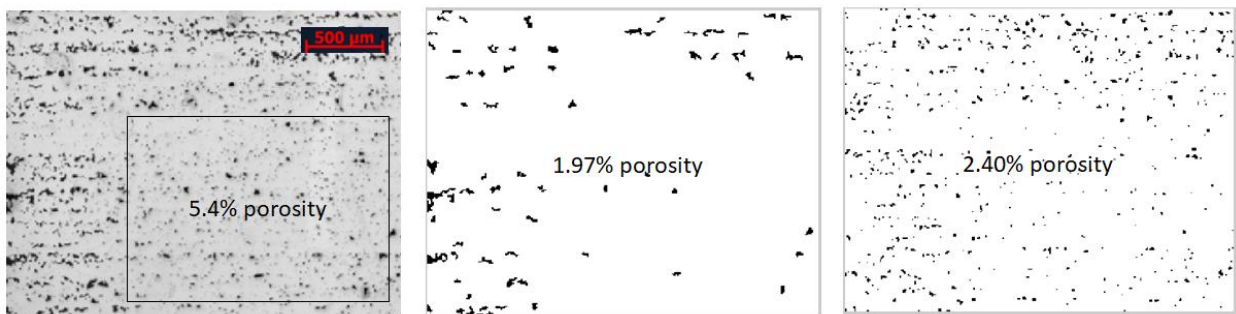
Figure 6.15 Porosity measurement (by optical pixel counting) for polymer binder printed part (Figure 6.12): core section only (5.4%), large pores (1.97%), and small pores (2.40%)
