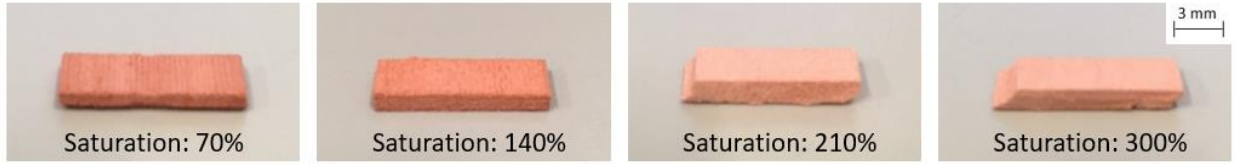
Figure 4.13 Sintered copper parts printed by the nanosuspension with different binder saturation ratios
