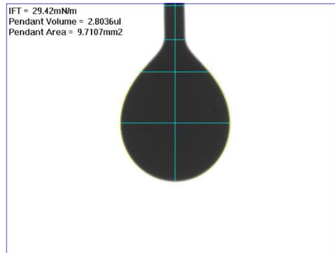
Figure 6.5 Pendant drop of 50% MOD ink, with a calculated surface tension of 29.42 mN/m
