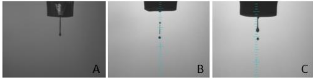
Figure 5.11 Inkjet testing of polymer binder (A), 15wt% (B) and 22.5 wt% (C) nanoparticle binder
