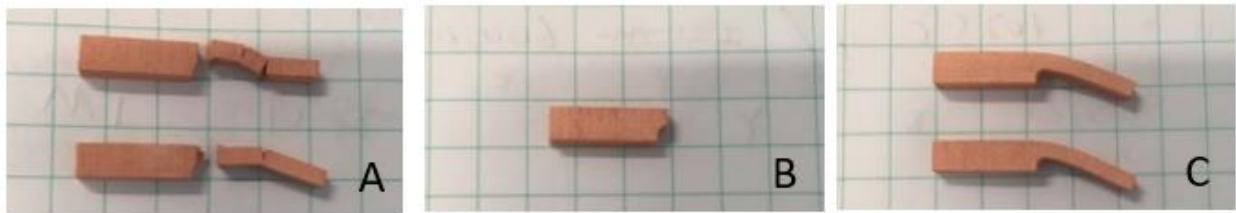
Figure 4.18 Overhang structure after sintering without supports, printed by: polymer binder printed with 100% binder saturation ratio (A), nanoparticle suspension printed with 70% (B) and 140% (C) binder saturation ratio
