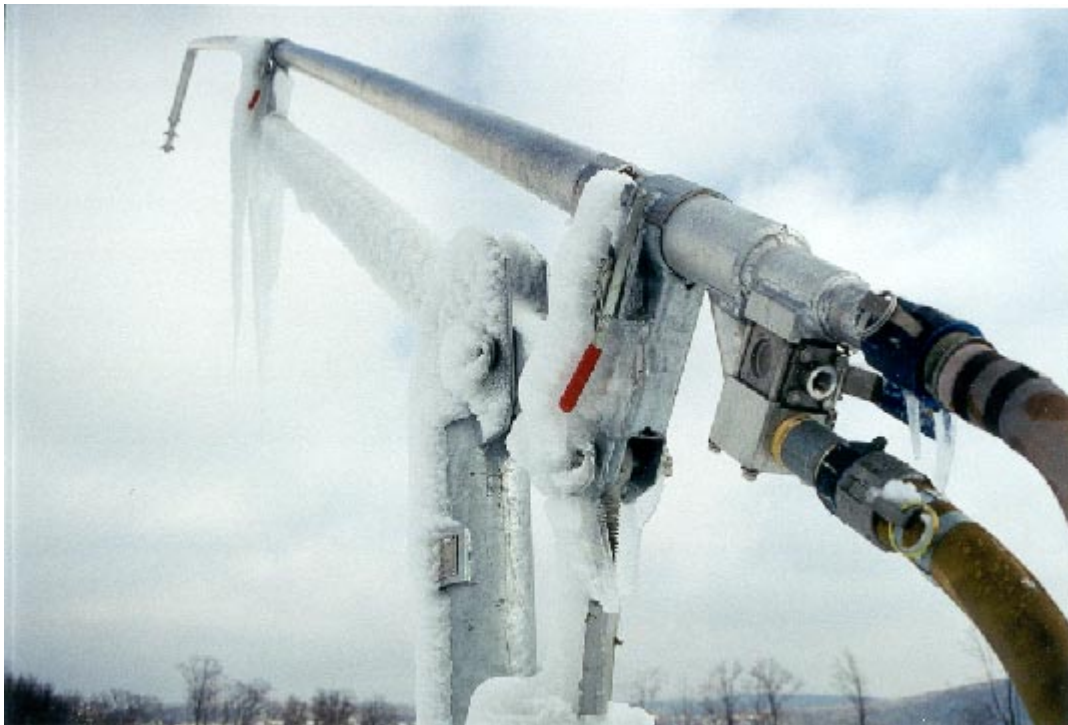
Figure 2.1 HKD Spectrum Snowmaking Tower
