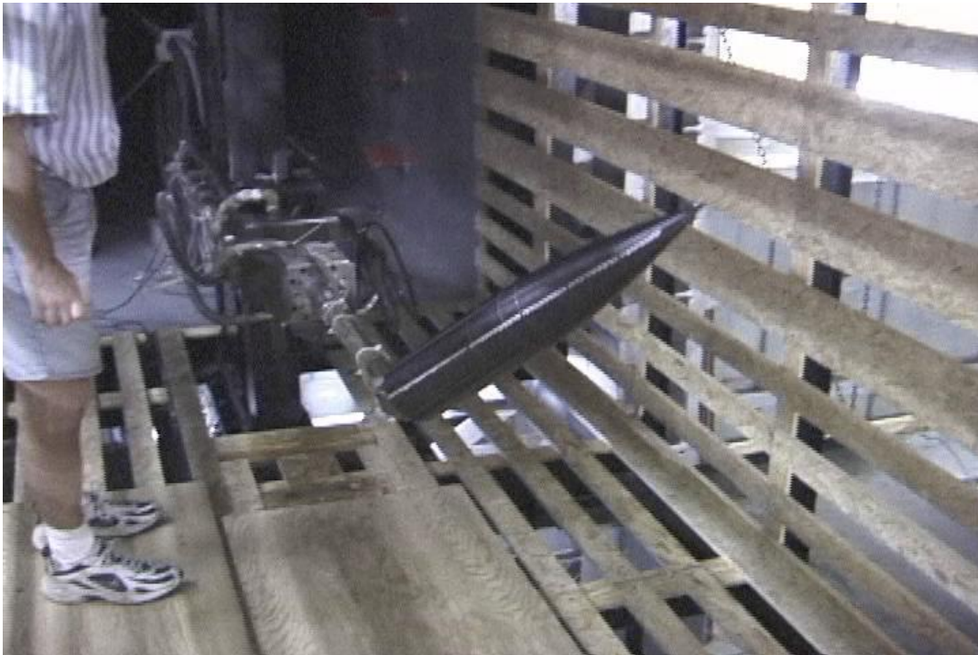
Figure 2.7 The DyPPiR Strut, Carriage, Pitch Actuator and Roll Actuator in the VPI & SU Stability Wind Tunnel with the D = 12.7 cm Stability Tunnel Model Installed. Note that Due to the Presence of the Pitch-Offset Block, the Model is at \approx 50^\circ with the Pitch Actuator Level, Allowing the Coning Motions to be Performed. Author Included for Scale.
