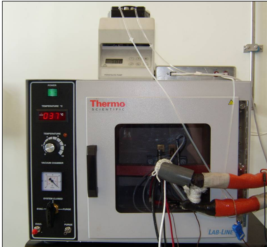
Figure 9. Vacuum oven during testing. DMFC test hardware depicted inside oven. Gilson peristaltic pump depicted on top of oven to the left. Methanol concentration meter depicted on top of oven to the right. Air flow lines wrapped in strip heaters enter oven through hole in front glass.
