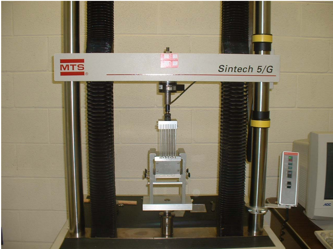
Figure 4.2 Sintech/MTS universal testing machine with Kramer shear press apparatus.
