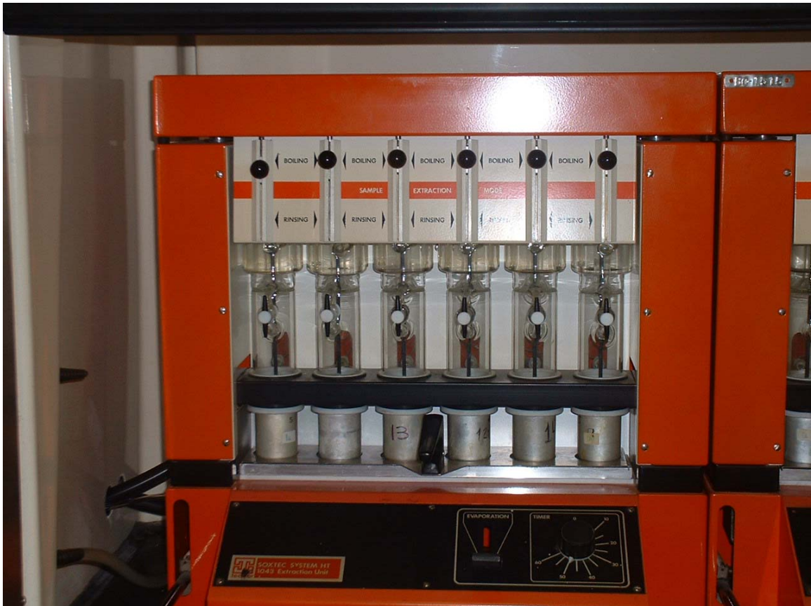
Figure 3.4 Soxtec extraction unit used to measure fat content.
