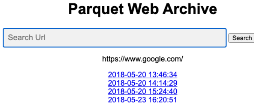
Figure 3.3: Demonstration web page for the response from a searched URL. In this example, we searched “https://www.google.com/” and the timestamp list below shows all the matching records in our collection.
