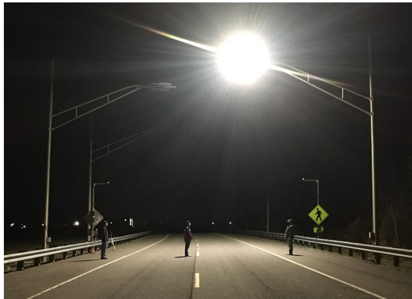
Figure 3. Photo. Crosswalk lighting design that was evaluated in the study.
