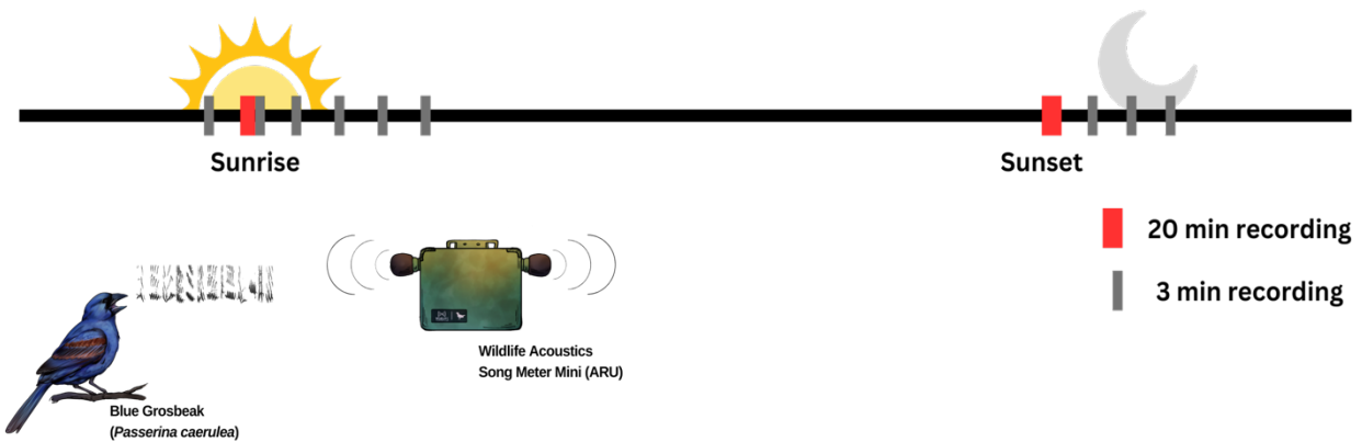
Figure 1.4: Passive acoustic monitoring daily schedule for autonomous recording units (ARUs) deployed at monitoring points across site treatments from May–June 2024 in southeastern Georgia. SongMeter Minis or SongMeter Mini 2s produced by Wildlife Acoustics Inc. (Maynard, MA, USA) were secured to a t-post 1.5 m off the ground and equipped with 2 omnidirectional microphones recording in stereo at a sampling rate of 44100 Hz with 18 dB of channel gain. Every ARU was configured to record daily with same schedule. ARUs recorded daily, for 20 minutes before sunrise in addition to 3 minute intervals every hour from 1 hour before sunrise until 4 hours after sunrise; and then record again for 20 minutes after sunset in addition to 3 minute intervals every hour until 3 hours after sunset. Altogether, 67 minutes of acoustic data were recorded daily at each monitoring point for 55 days.
