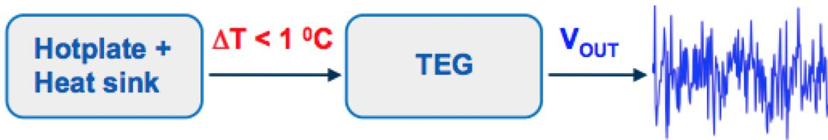
Figure 3.5: Block Diagram of TEG Random Number Generator.
