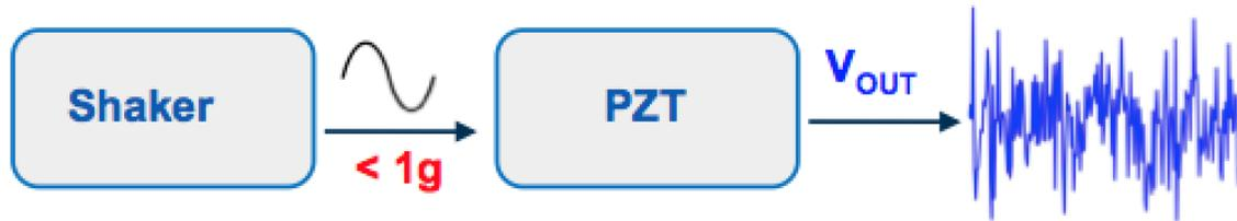
Figure 3.4: Block Diagram of Piezo Random Number Generator.
