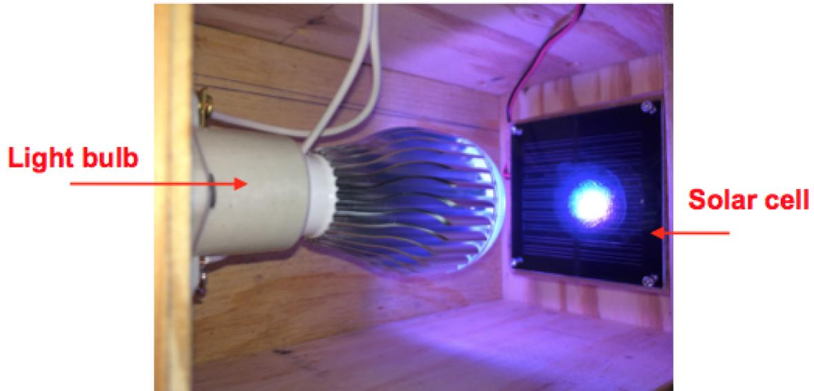
Figure 4.5: PUF Testing Setup of Solar Cell.
