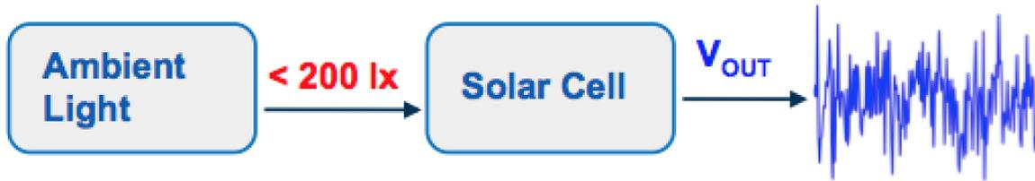
Figure 3.6: Block Diagram of Solar Cell Random Number Generator.
