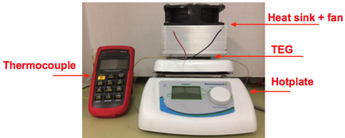
Figure 4.3: PUF/RNG Testing Setup of Thermoelectric Generator.
