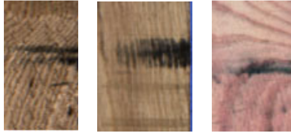
Figure 8.3 Typical surface stains
