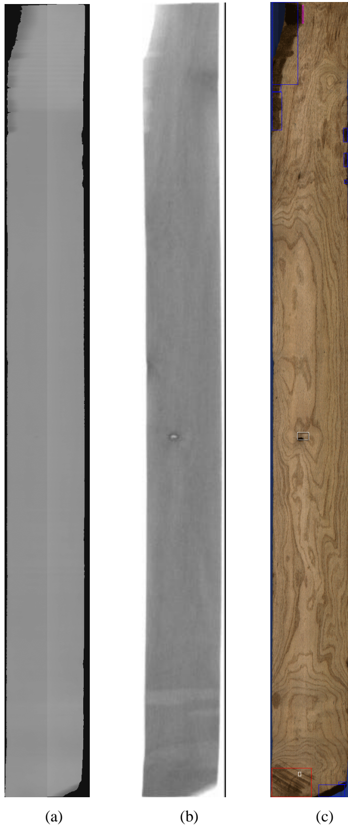
Figure 9.2. The laser, X-ray and color images of a board that contains wane/thin board.
