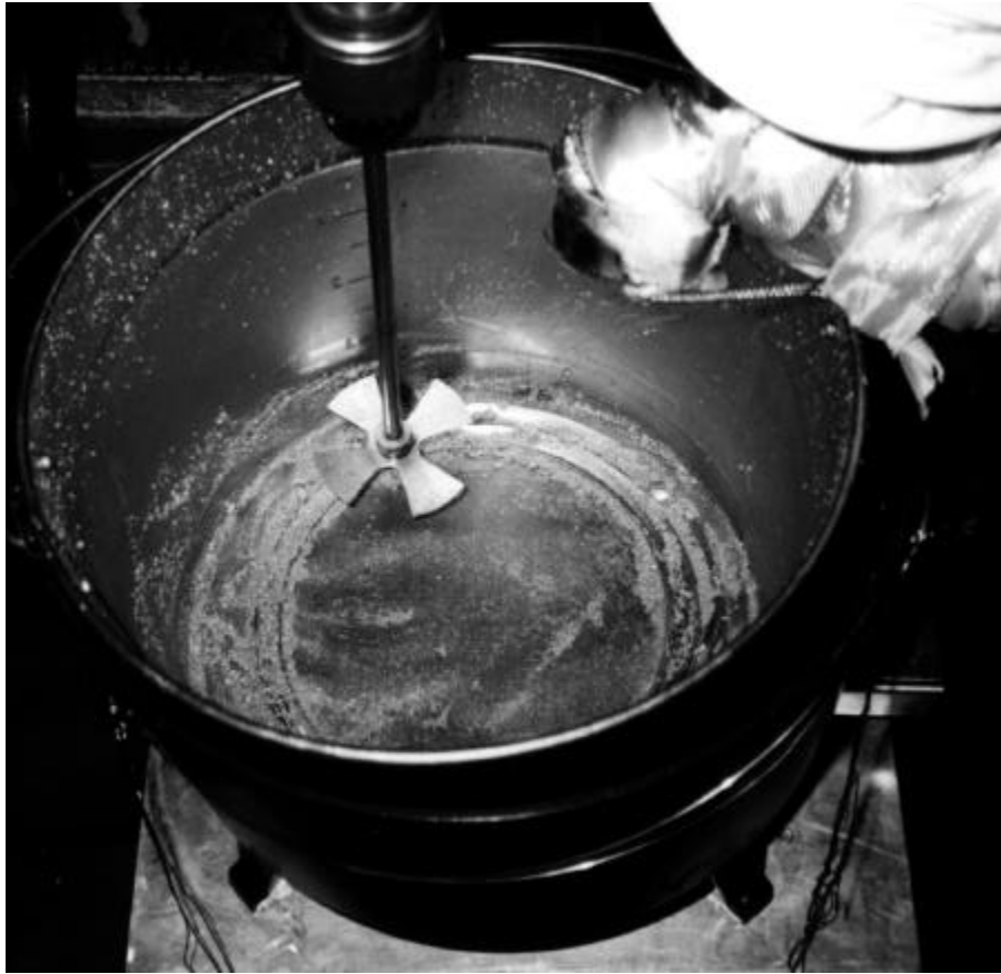
Figure A.4 Close-up of the Mineral Oil Dissolution Process that shows the Impeller and the Screening System with leftover Reclaimed HX8000 Pieces.
