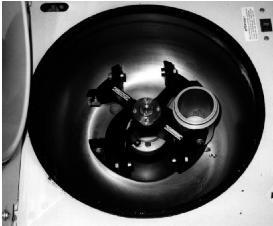
Figure A.5 Fisher Scientific Marathon 21K/R Centrifuge used to separate the pieces of Reclaimed HX8000 from the Mineral Oil, the Kerosene, and the Hexanes.
