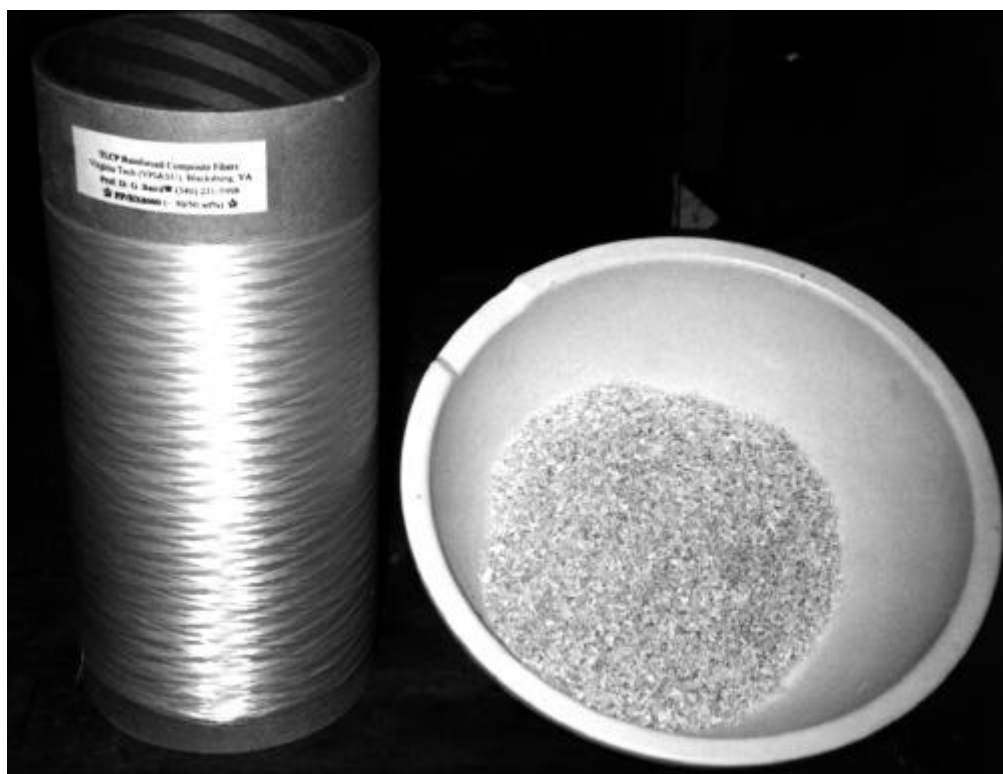
Figure A.2 Spool of Composite Fiber (40 wt% HX8000 / 60 wt% PP 6523) that was generated in the Dual Extrusion Process and the Granulated Pieces for Reactive Extrusion.
