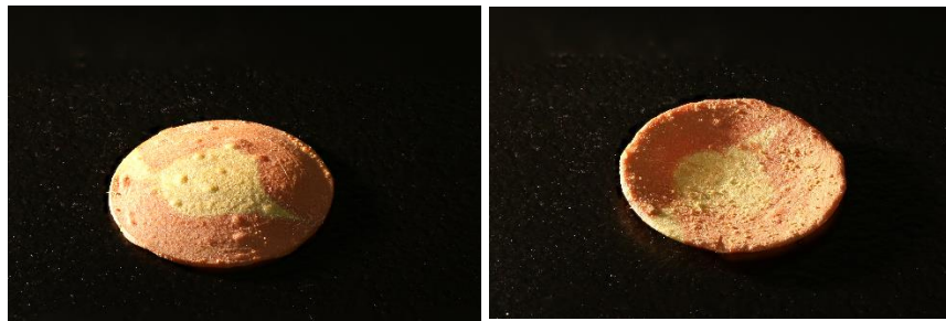
Figure 23. Sintered HIFU Transducer element
