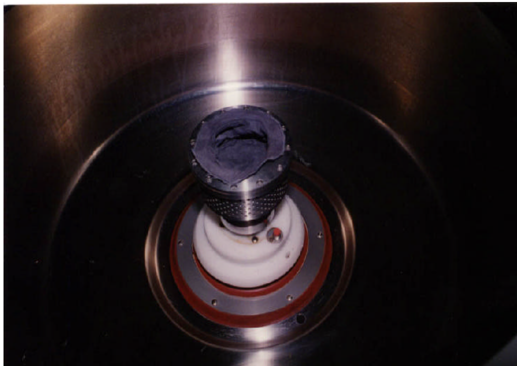
Figure 3.2. Lab-scale screen bowl centrifuge.
