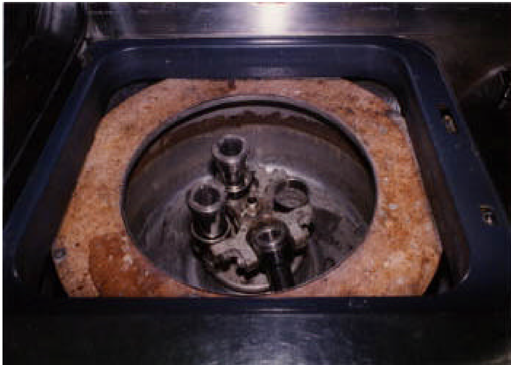
Figure 3.1. Lab-scale solid bowl centrifuge unit.
