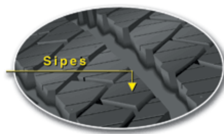
Figure 10. Representation of sipes on tires
