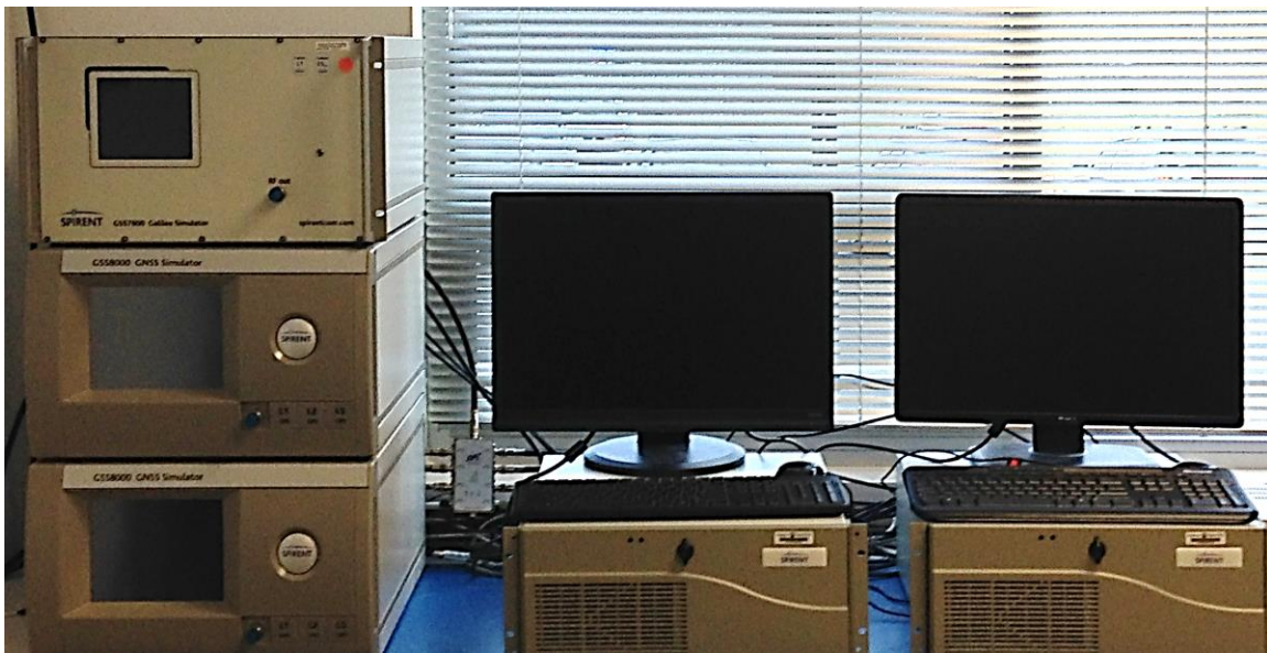
Figure 4: Spirent GNSS 8000 hardware RF signal simulator used in the study
