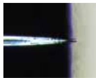
Microneedle penetration of ex vivo porcine skin.
