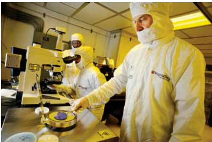
Materials are controlled with single atomic layer precision. A key enabling tool for deposition of subnanometer dielectric layers is the so-called Atomic Layer Deposition chamber seen in the forefront.
