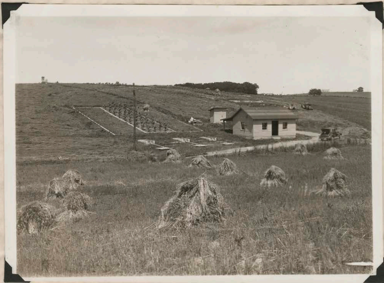
This picture gives a general idea of the field setup for the soil and water conservation research project. All of the field laboratory work is done in this field house which was constructed especially for that purpose. To the left of the field house is the series of three plots on 20% slope. The automatic rainfall recorder and the recording thermometer cage can be observed in the upper left corner of the picture.
