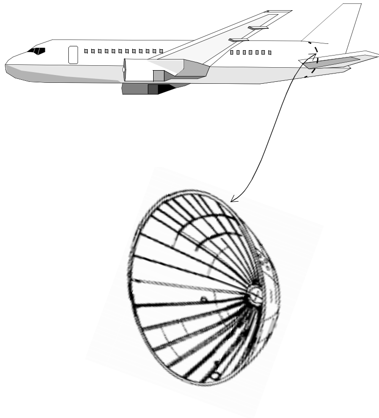
Fig. 1.1 Aft Pressure Bulkhead on a Large Transport Airplane
