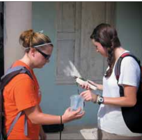
Students use a handheld sensor to detect contaminants in the water supply in the town of Verón.
