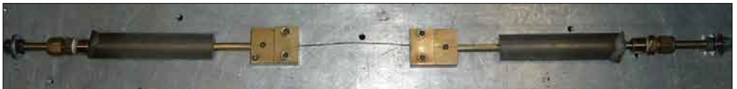
Figure 4. Geometry of electrodes inside the vacuum chamber, shown with copper fuse
