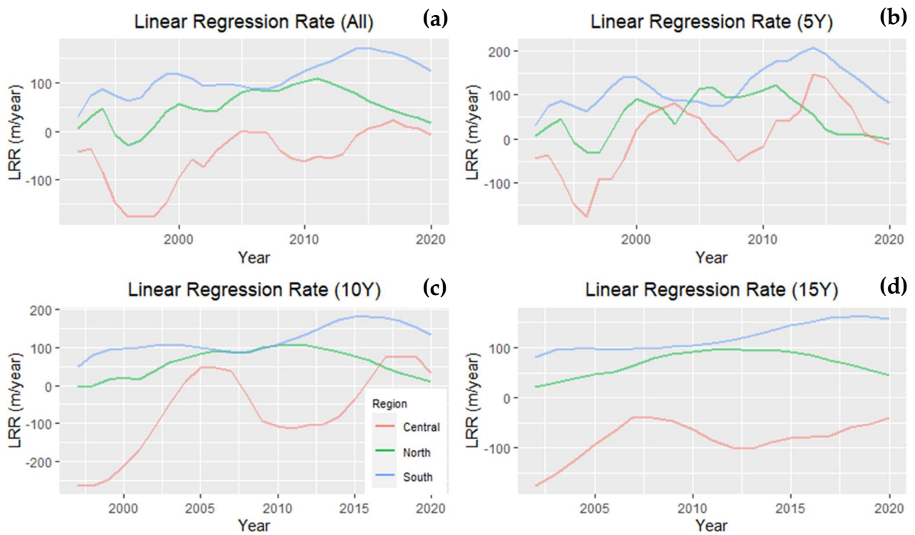
Figure 4. Linear regression rate of shoreline movement over time and space: (a) average of all time depths, (b) 5 years' time depth, (c) 10 years' time depth, and (d) 15 years' time depth. In the figure, positive values indicate erosion and negative values indicate accretion.
