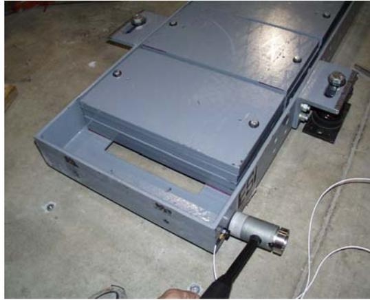
**Figure 3.30 (cont.) – PTMD Modal Testing: Lateral Mode**
