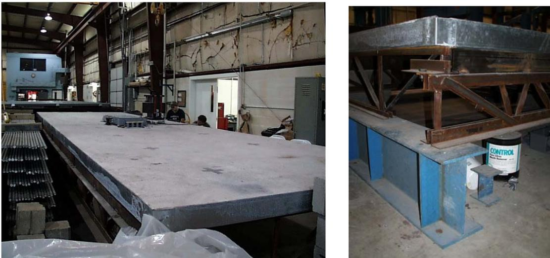
**Figure 3.3 – Experimental Floor (left) and End Condition (right)**
