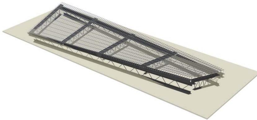
**Figure 3.23– Third Mode (Torsional Mode)**
