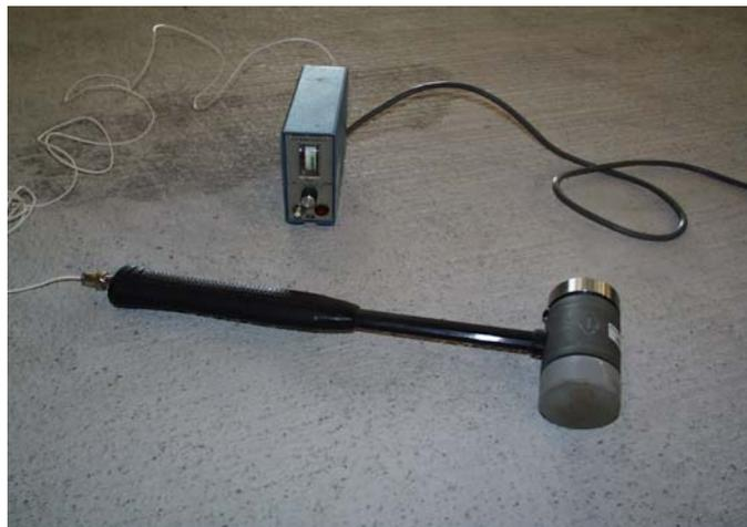
**Figure 3.9 – PCB Impulse Force Hammer**
