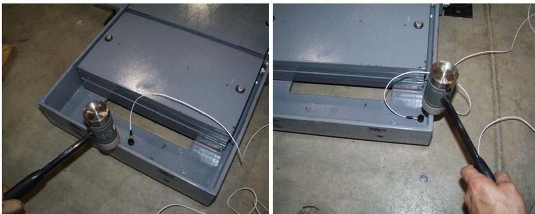
**Figure 3.30 – PTMD Modal Testing: Bending Mode (Left) and Torsion Mode**
