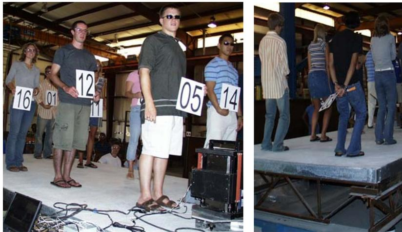
**Figure 3.37 – Humans on Experimental Footbridge Standing Straight Leg (Left), Standing with Legs Bent (Right)**
