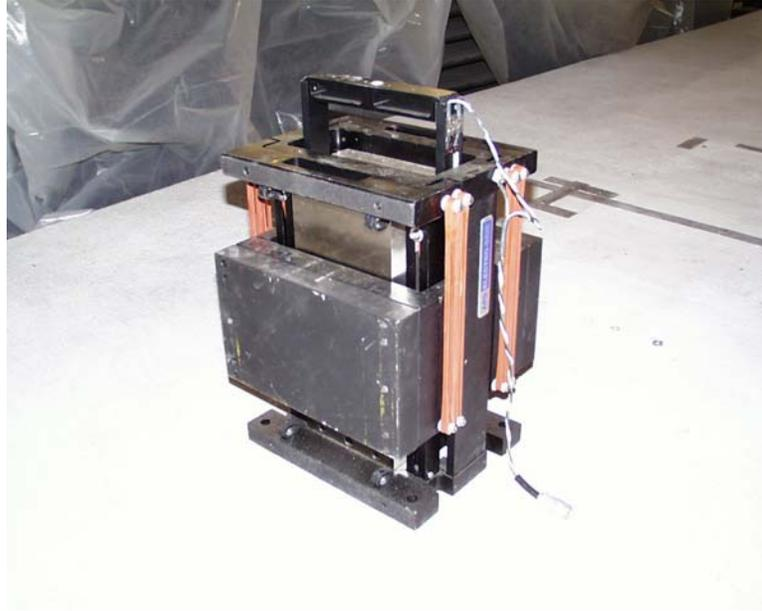
**Figure 3.10 – APS Electro-Seis, Model 400 Shaker**
