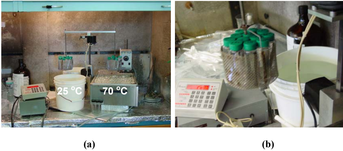
Figure 2-2. Photographs of the cyclic thermal testing apparatus. (a) Rotating assembly and water baths, (b) basket holding glass vials that contain bonded specimens immersed in solutions.
