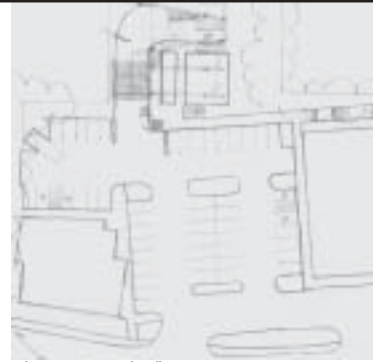
advantage: central walkway disadvantage: column displacement
