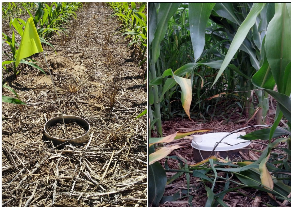
Figure 2. Metal ring after field installation at the pre-sampling (left) and at the sampling and post-sampling stage (right).
