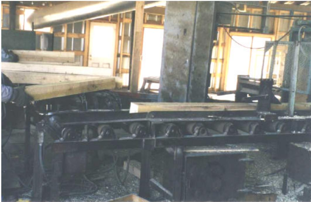
**Figure 12. Quality Cant Sections Entering a Circle Gang Ripsaw in a Typical Pallet Manufacturing Plant**
