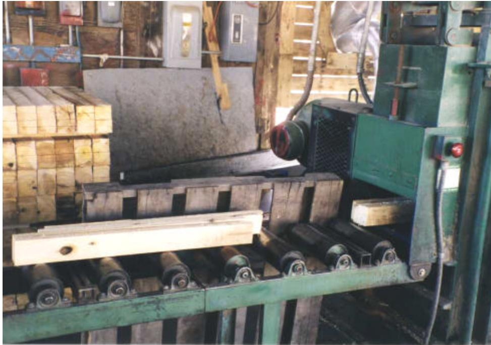
**Figure 13. Pallet Parts Exiting a Circle Gang Ripsaw in a Typical Pallet Manufacturing Plant**
