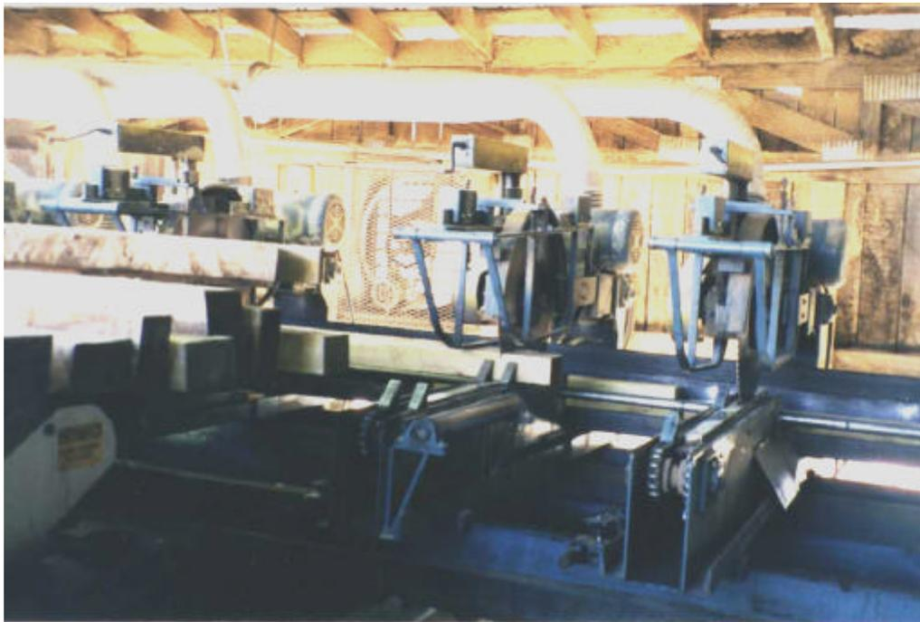
**Figure 10. Hardwood Cants Entering the Trim Line of a Pallet Part Sawing System**
