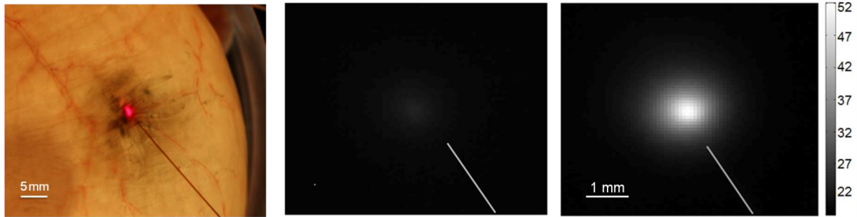
Figure 18: Irradiation from light-guiding, hollow-core microneedle after delivering SWNHs into the inflated bladder wall. Left) photograph showing microneedle position (Note: the red guide laser is visible), Middle) thermograph of non-infused control, Right) thermograph of SWNH perfused tissue. Color scale is in Celsius, white lines denote fiber path.
