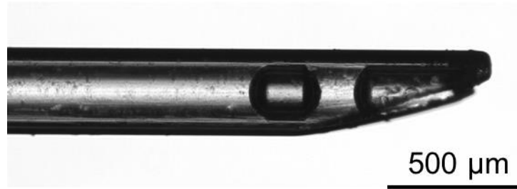
Figure 11: Image of sharp, beveled tip of An FMD. Water is visible inside the hollow bore.
