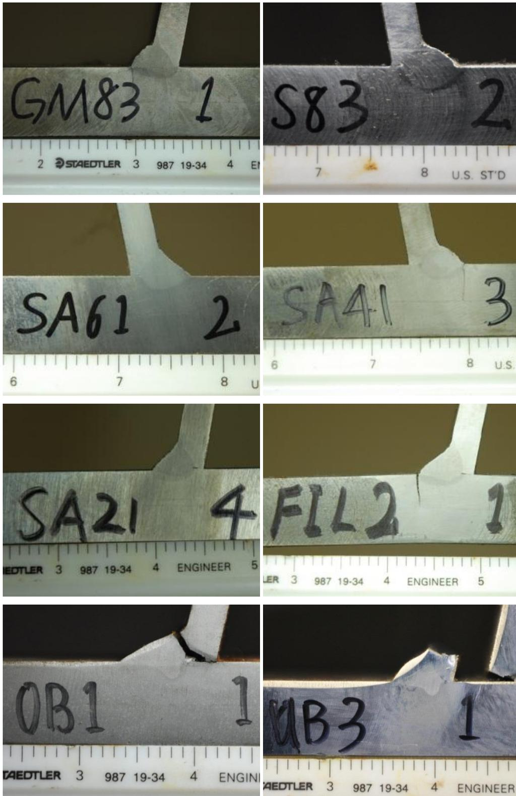
Figure 3.4 Typical weld profile in each series
