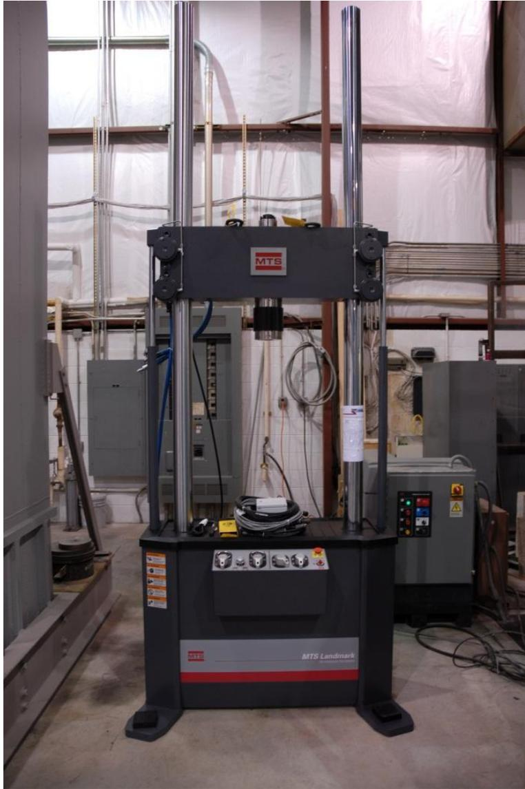
Figure 3.8 MTS servohydraulic test system at VT
