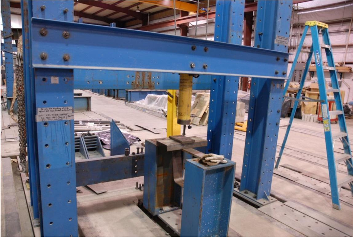
Figure 3.22 Setup for breaking specimens from fatigue cracks
