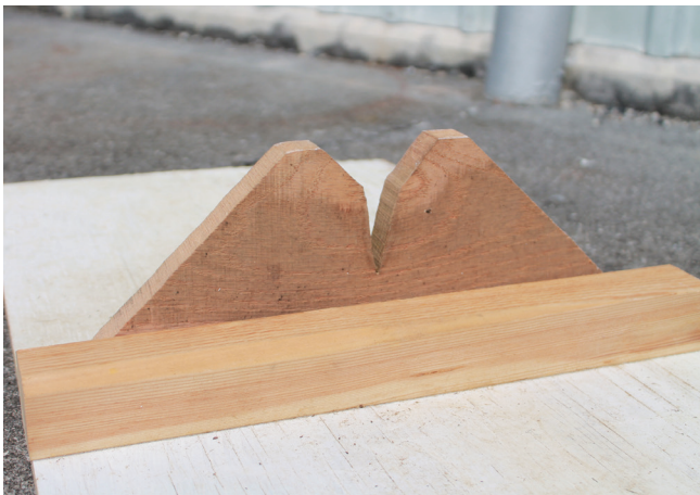
Figure 1: Wooden pod stripper used at Virginia Tech's Kentland Farm for edamame pod separation.
