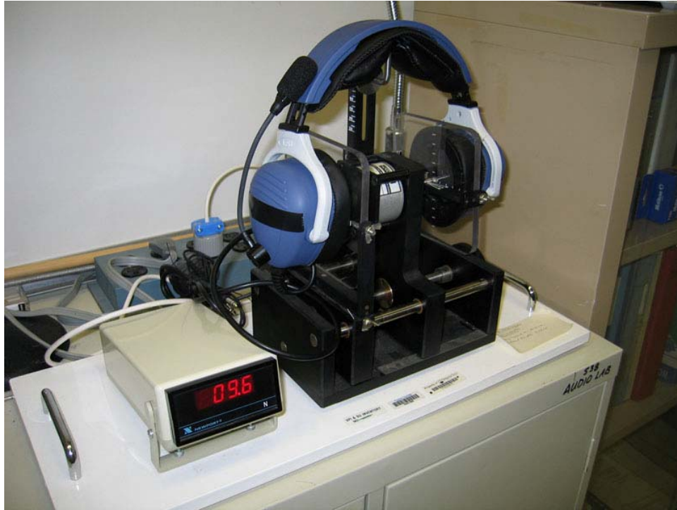
INSPEC earmuff headband force measurement apparatus.
