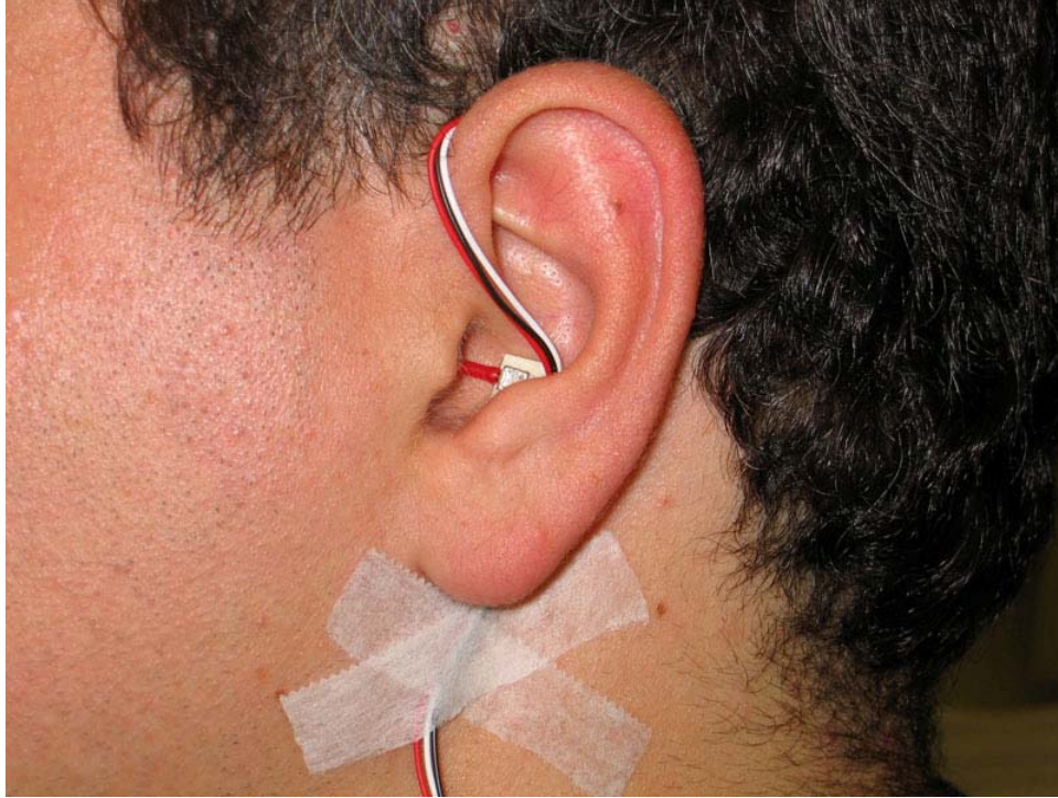
Deep microphone (left ear only) in proper testing configuration.
