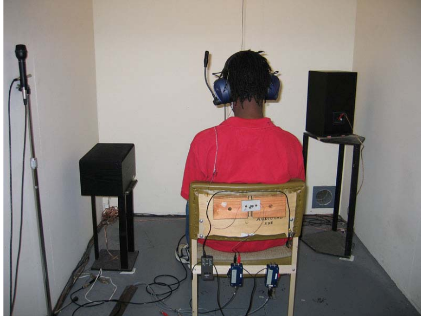
Figure 18. Interior view of the reverberant chamber with seated subject.
