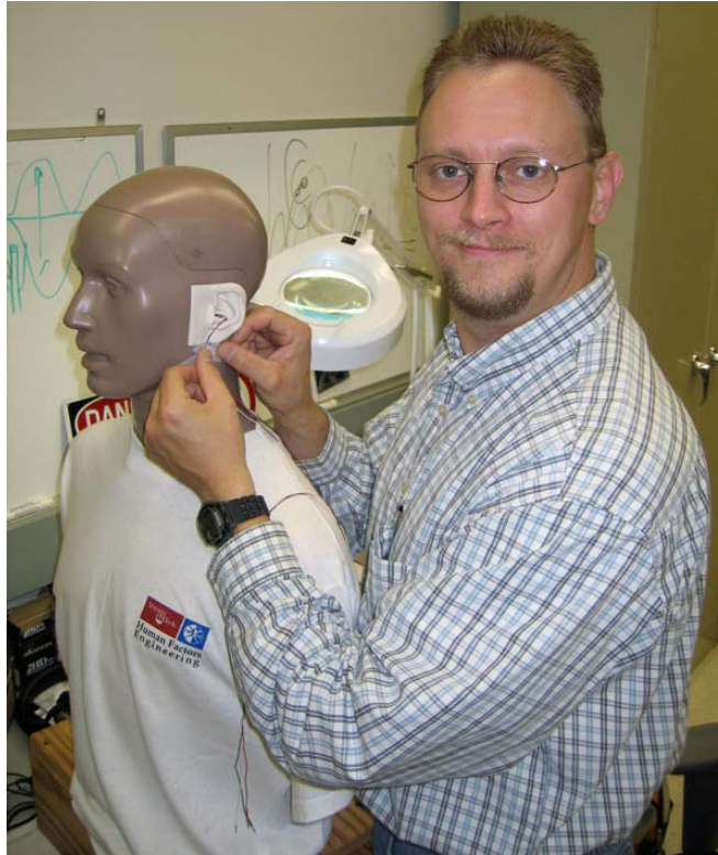
Pre-testing microphone fit and function using artificial test fixture (ATF) manikin.
