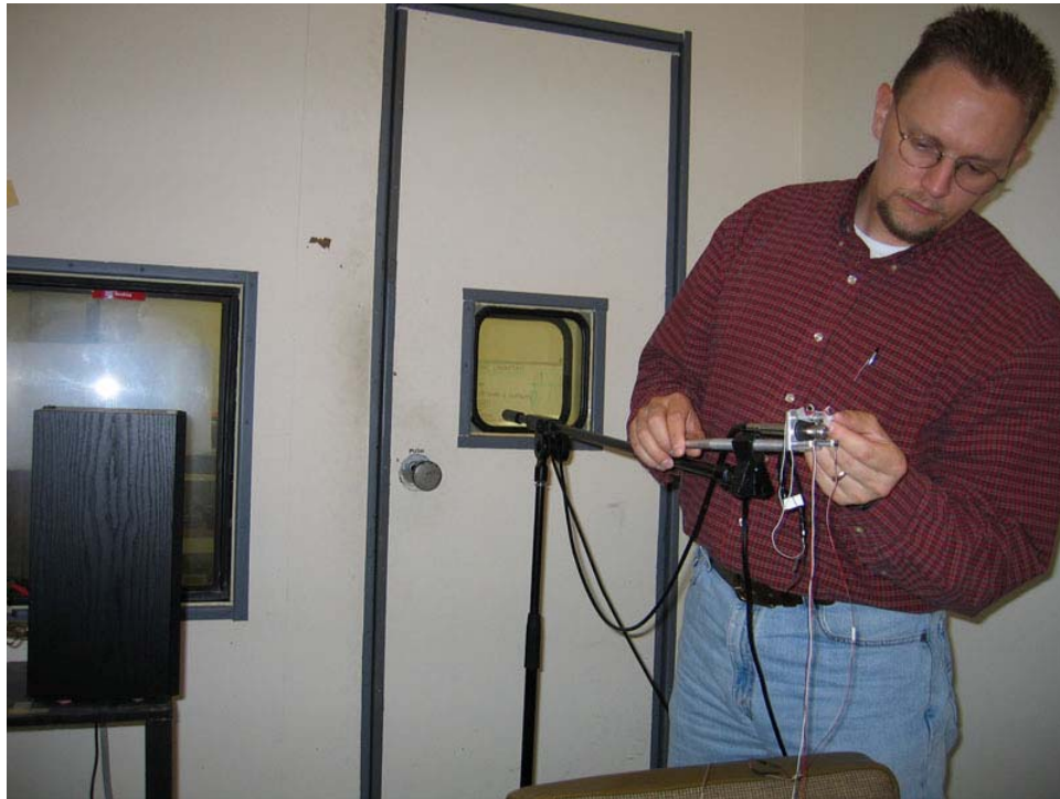
Setting up miniature microphone calibration test fixture centered inside reverberant chamber.
