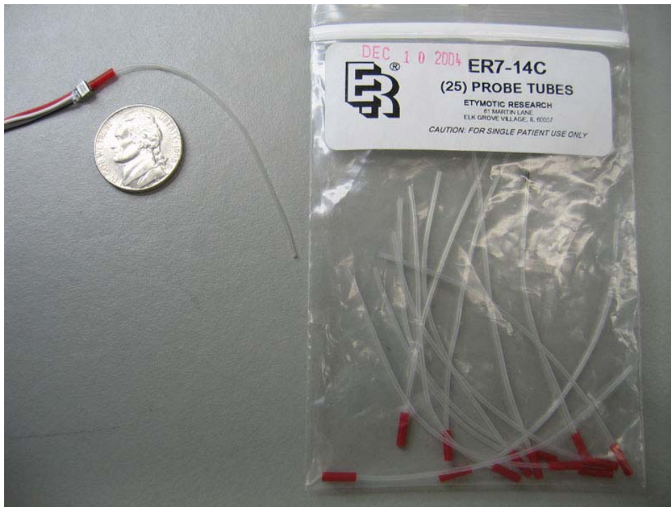
Deep probe tube microphone with probe tube attached and extra probe tubes.
