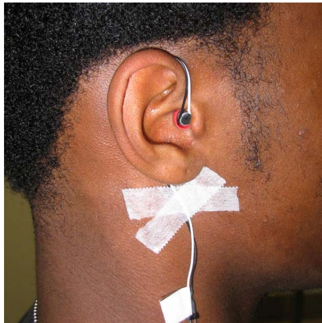
Shallow microphone (right ear) in proper testing configuration. Left ear microphone configured the same.
