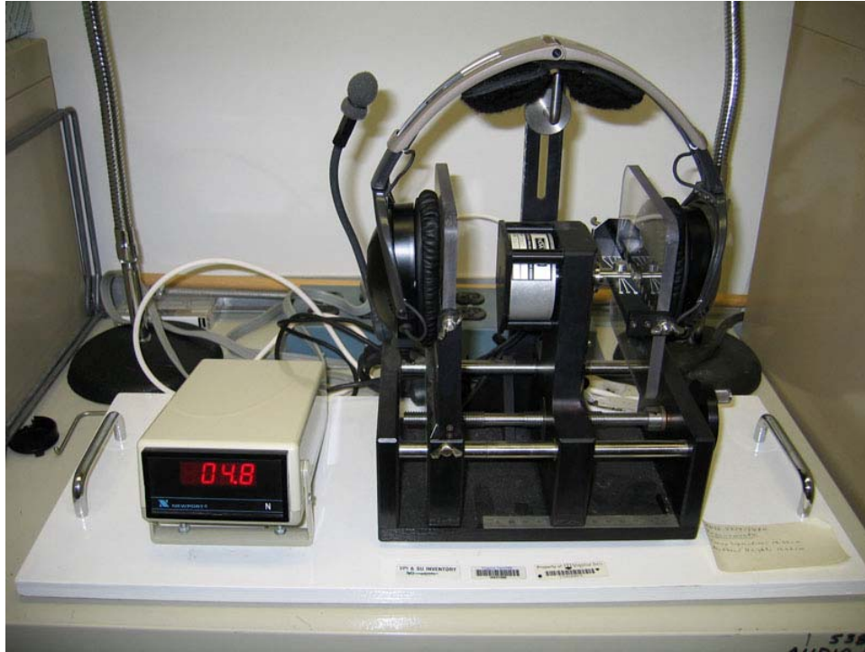
Figure 16. INSPEC earmuff headband force measurement apparatus.
