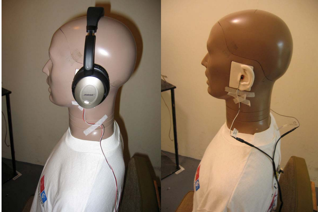
Pre-testing in-concha microphone (left) and shallow microphones (right) with and without sample headset on ATF manikin.
