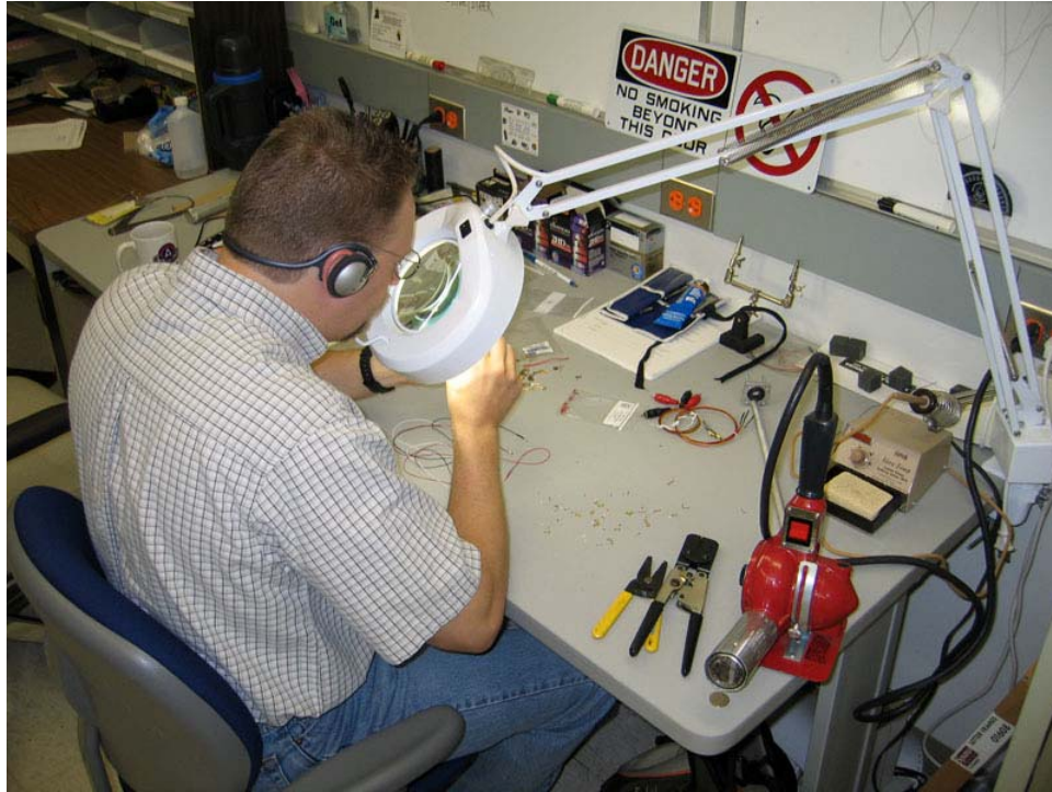
Adding pin-connectors to the miniature microphone wires.
