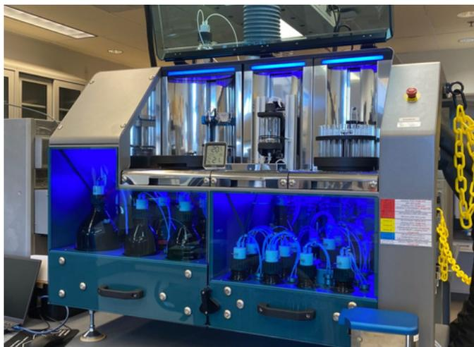
*GlycoMIP houses the only two commercially available Automated Glycan Assembly instruments in the United States. The Glycoconeer instruments can rapidly produce glycans and help drive the field of glycoscience forward.*
