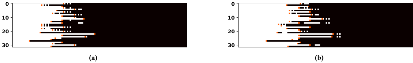
Figure 5. Bitmap visualization of timing failures in FPGA paths: how logic 1 (white) propagates through 32 paths in two different FPGAs (same design), changing the preset values (black) from left to right. Red dots indicate the first failing locations in each path.
