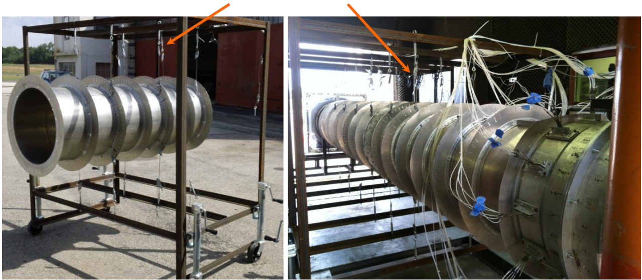
Figure 8. Tunnel section turnbuckle support system. Photos by Author, 2013.
