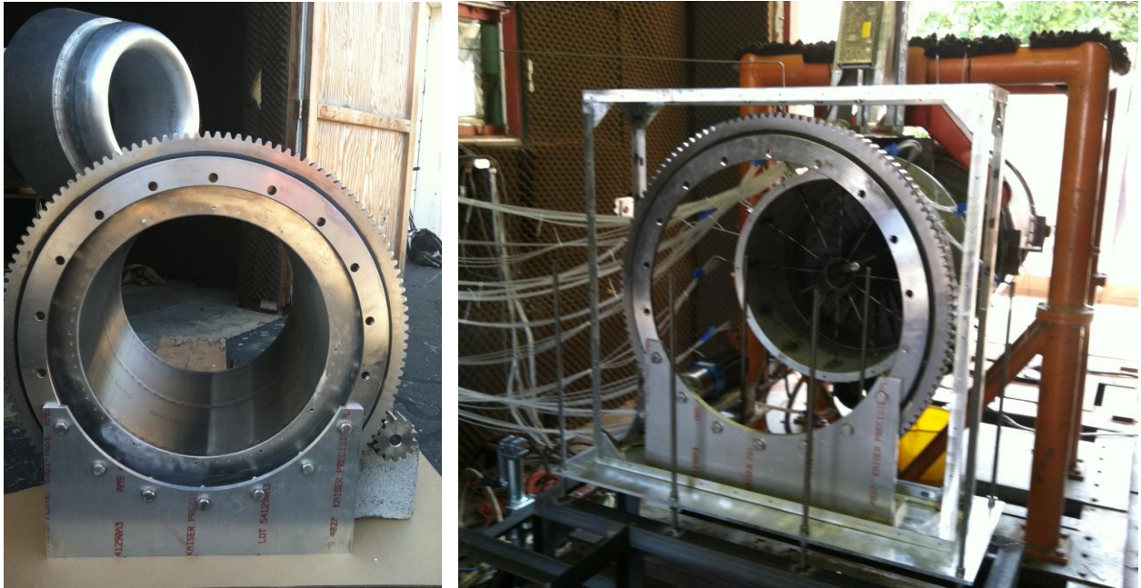
Figure 6. Photographs of distortion screen support rig and bearing (left), and support stand assembly (right). Photos by Author, 2013.
