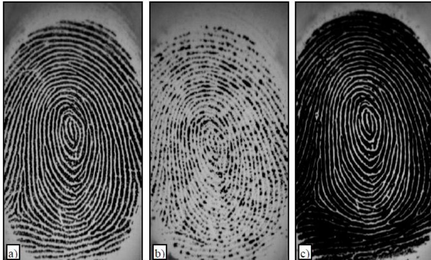
Figure 2.2. Three fingerprint images of the same finger with different skin conditions acquired with an optical FTIR scanner: a) normal, b) dry, c) wet [from Maltoni et al., Handbook of Fingerprint Recognition (2nd Ed.) (2009)] [1]
