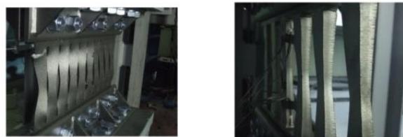
Figure 3. The cyclic behavior of steel dampers [22]
