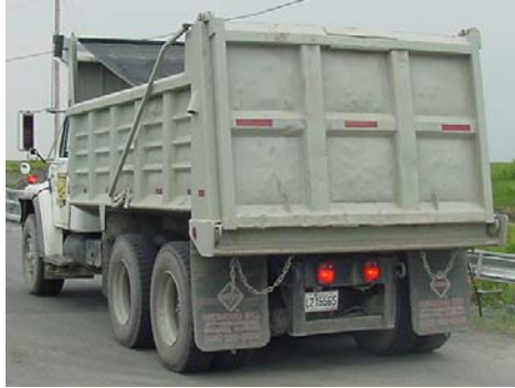
Figure 15. Three-Axle Dump Truck Used for Shenley Bridge Live Load Testing
