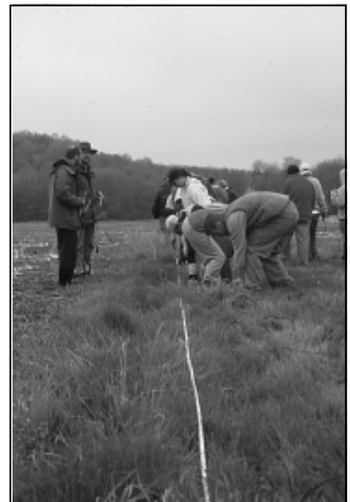
TA Jamie Buscher (far left) and Dr. John Hole (2nd from left) supervise installation of seismometers into the ground for a seismic refraction survey of a New River terrace at Kentland Farms
