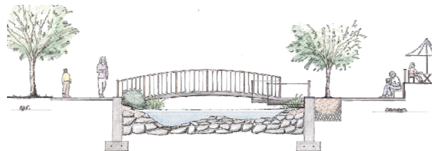
2-Year Storm Event (approximately 150 cfs)
