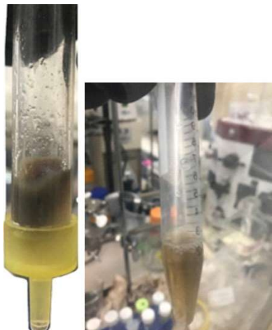
Figure 3.6. Pictures from an ANME-1 purification. Left: Ni-resin after application of protein sample turns brown. Right: concentrated protein in solution is also brown. This is an indication of good iron-sulfur incorporation in the protein as it is expressed in E. coli .
